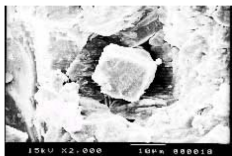
Fig. (3) : SEM shows salt crystals form whiskers filling secondary micropores and coats its texture
