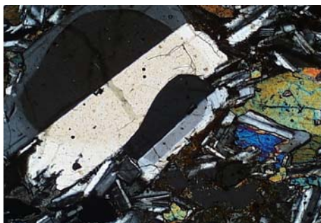
Fig. (5): Polysynthetic lamellar twinning of plagioclase phenocrysts in basalt sample. Cracks are also observed.
