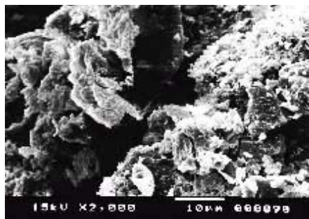
Fig. (4): SEM micrograph shows that the minerals are fractured and the resulting fragments are separated by open transverse fractures.
