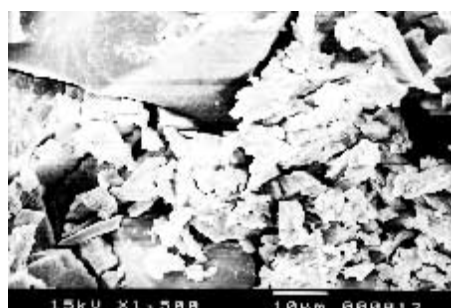
Fig. (4): SEM shows that most mineral grains are loosened from each other
