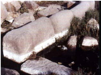
Fig. (3): Field view showing parts of basaltic blocks immersed in domestic water. Salt efflorescence can be noted
