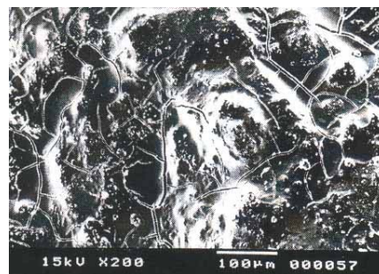
Fig. (6): SEM micrograph shows a different cracks in slieaster A.R after artificial weathering.
