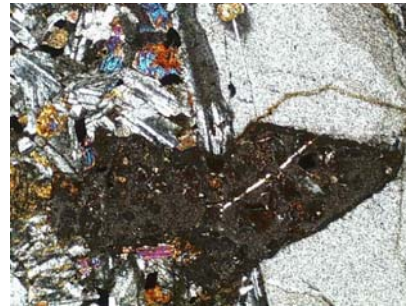
Fig. (2): Fractures and fissures in the internal Structure and the formation of clay minerals as secondary alteration.
